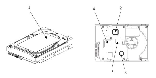
Figure 4.5 Surface temperature measurement points
